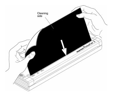
FIGURE 18. Cleaning the platen roller.
